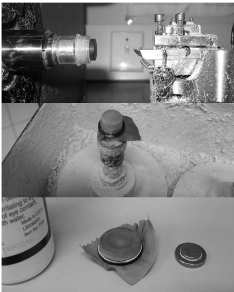
Figure 3. Stages of RGP CL manufacturing process – diamond turning and polishing.
