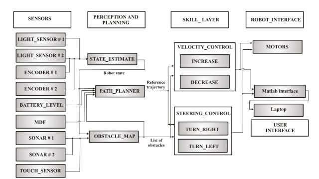
Figure 5. Proposed hybrid control architecture
