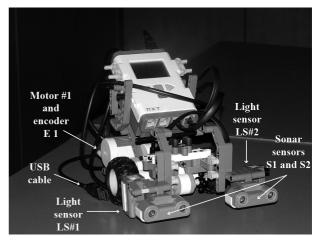
Figure 6. Mobile robot built on LEGO Mindstorms NXT Technology
