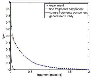
Figure 3. Fine and coarse fragments components of the generalized Grady distribution fit of the experimental data (projectile 1 [19])
