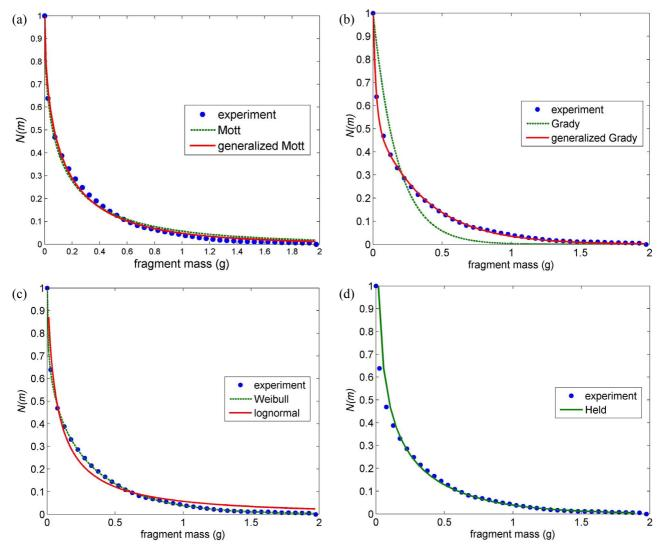
Figure 1. Comparison of the relative cumulative fragment number experimental data for projectile 1 [19] with: (a) the Mott and the generalized Mott, (b) the Grady and the generalized Grady, (c) the Weibull and the lognormal and (d) the Held fragment mass distribution model
