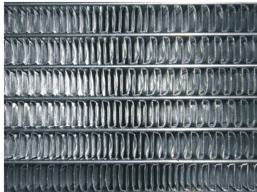
Figure 5. Air side segment of microport tube / louver fin R744 heat exchanger
