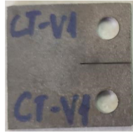
Figure 2. An example of a CT specimen (code name, CT-VT1).
