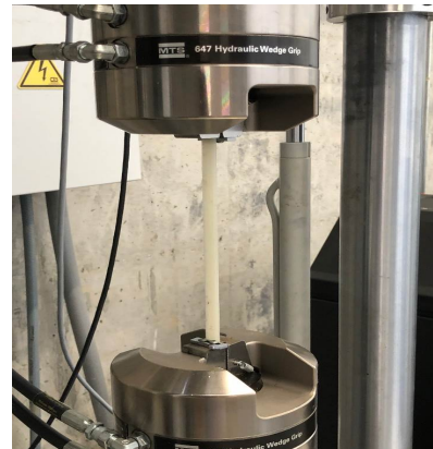
Tensile test of the specimen made of composite material in a universal testing machine
