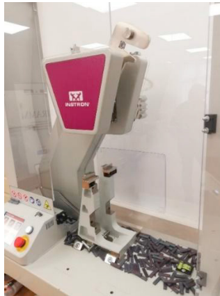
Fig. 2. Instron CEAST 9050 Charpy instrumented pendulum.
