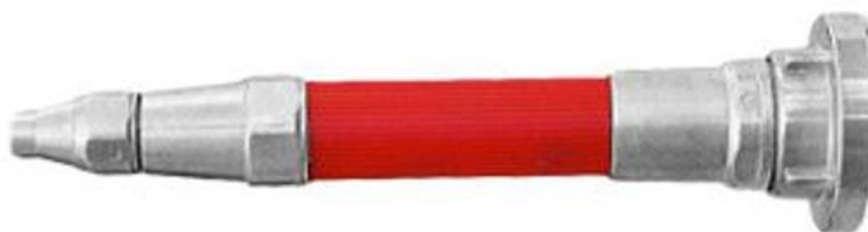
Figure 1. Standard hydrant nozzle (orifice diameter 16 mm, hose connection flange Ø75mm - type B, length 410 mm, height 126 mm, weight 1.75 kg)
