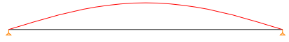
Fig. 2b First Mode Shape for the Tube, Simply Supported at Both Ends, f_{01}=1.06\text{Hz}
