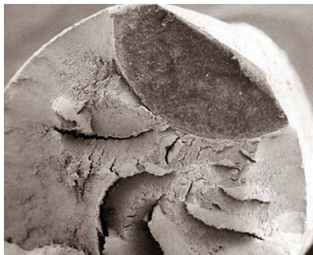
Slika 7. Zamorna prslina nastala na mestu dodira žice sa koturačom Figure 7. Fatigue crack initiated at the contact point with a sheave
