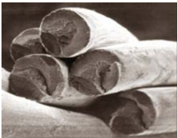
Slika 6. Zamorne prsline na mestu kontakta pojedinačnih žica. Inicirane prsline se vide nakon kidanja struka zatezanjem Figure 6. Fatigue cracks at the contact points of individual wires. Initiated cracks are visible after fracture of strand in tensile test
