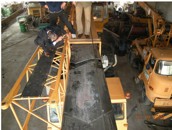
Figure 3: Segments preparation for auto crane repair
