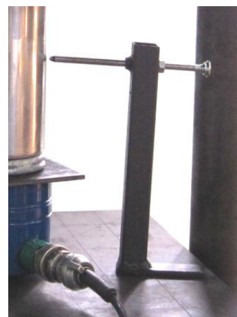
Fig. 4: Mechanism for making dents
