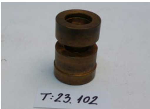
Figure 6. Model of Tesla's radial bearing for electric motors, T:23.102 (Collection of Objects from the Field of Mechanical Engineering)
