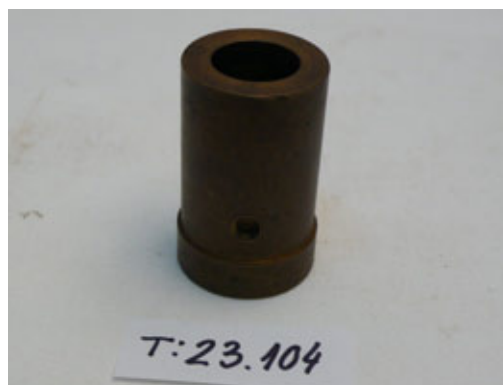
Figure 5. Machined piece for slide bearing T:23.104 (Collection of Objects from the Field of Mechanical Engineering)
