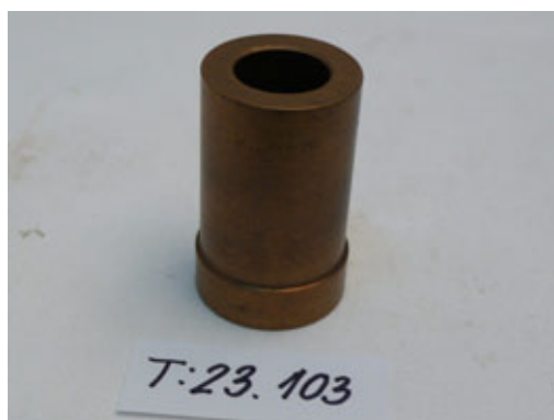
Figure 4. Machined piece for slide bearing T:23.103 (Collection of Objects from the Field of Mechanical Engineering)
