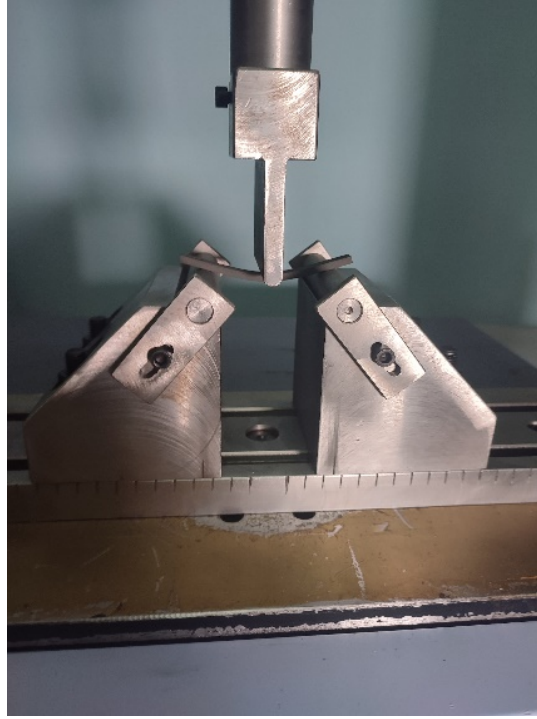
Fig 4. Shimadzu AGS-X Universal Testing Machine with a Specimen and 3-Point Bending Test Tool.
