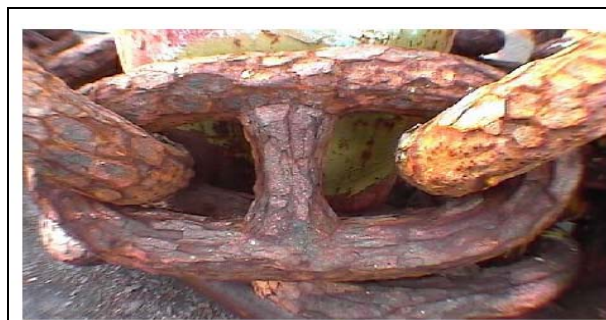
Slika 5. Korozija lanca brodskog čekrka /10/ Figure 5. Corrosion of chain of ship windlass /10/
