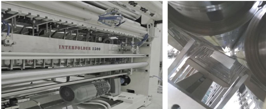
Fig. 16.4 Upgraded machine INTERFOLDER 1500, left: front view from where the paper enters, right: section for folding and folding wipes
