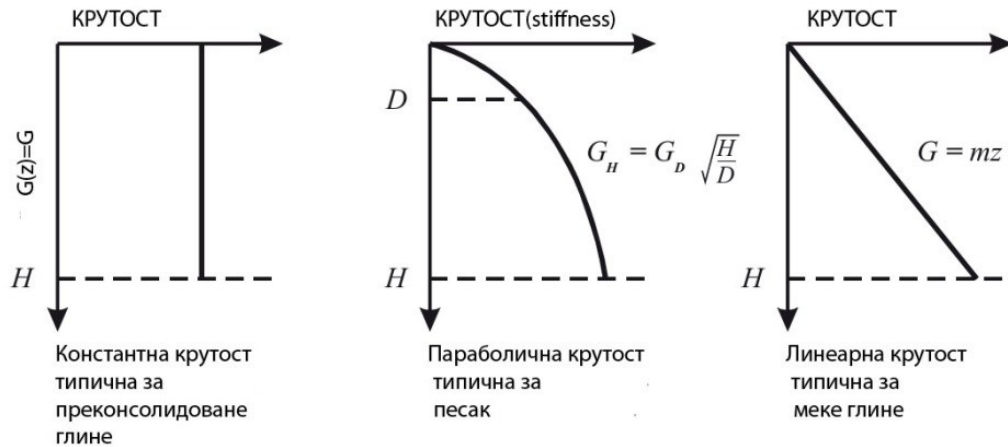
Figure 1. Typical stiffness profiles for foundation strata a) Constant Stiffness (Typical of overconsolidation clay) b) Parabolic stiffness (Typical of sand), c) Linearly increasing stiffness (Typical of soft clay)
