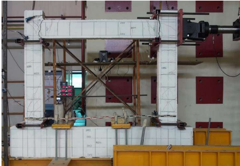
Fig. 4. Cracking pattern of the steel X-braced RC frame at the end of the test [12,13].
