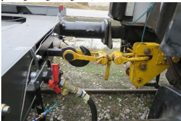
Figure 2. Special hook installed on the passenger wagon
