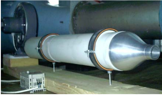
Figure 2. Open air tunnel for hot-wire probe calibration. Pipe and diffusor are made of hard plastic, nozzle of duralluminium.
