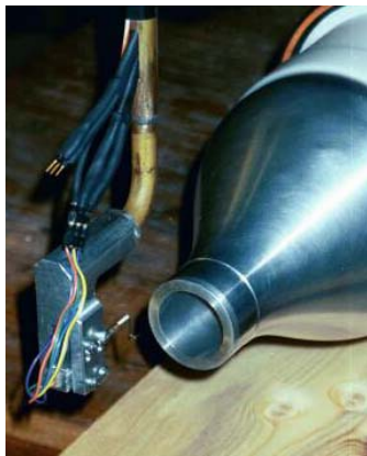
Figure 5. VP-2vs probe static calibration in the tunnel air jet
