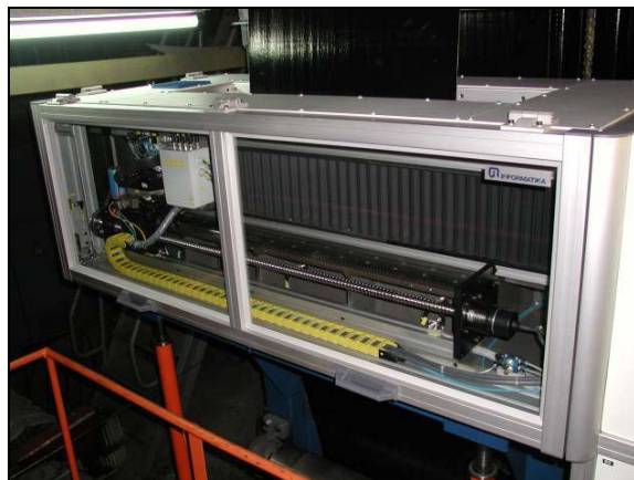
Figure 6. Prototype measuring station designed for post-calender thickness measurement of rubberized steel cord (the system was installed in Belshina tiremaking company, Belarus). Measuring module (up) and complete measuring station (down).
