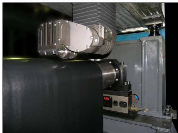
Figure 8. Prototype of measuring station designed for post-calender thickness measurement of rubberized textile cord (installed in AMTEL Voltair tiremaking company, Russia); Robotic arm module (up), traversing subassembly (center), and measuring module+reference roller with embedded RCS tension sensor and angular encoder (down).
