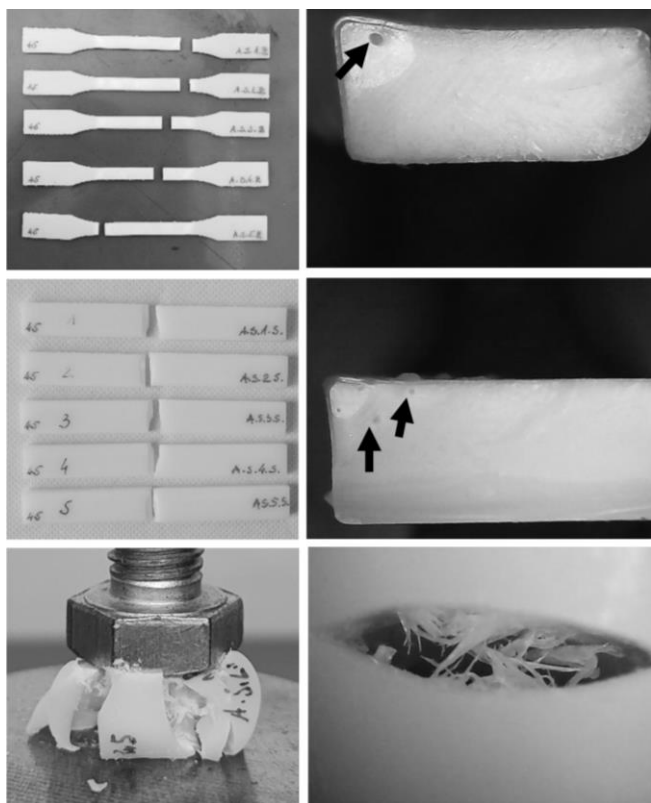
Figure 4. Left: fractured SLA printed specimens; right: fractured surfaces after tensile (first row), three point bending (second row), and compression (third row) testing.
