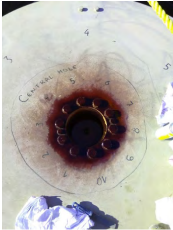
Figure 7 Critical places on the top holder for blades after spraying penetrant-evaluation of surface irregularity
