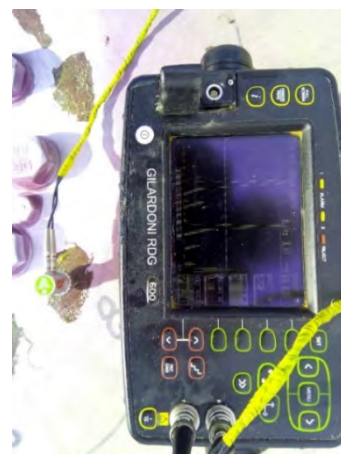
Figure 12 Critical area holder-reducer assessment of volume irregularities by conventional ultrasound method
