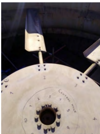
Figure 5 Top blade holder with blades-Top view (critical places are marked with the numbers)
