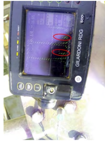
Figure 10 Critical place holder-blade evaluation of volume irregularity by using conventional ultrasonic method
