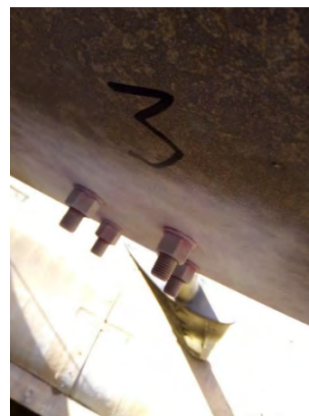
Figure 6 Critical places on the down holder for blades after spraying developer-evaluation of surface irregularity
