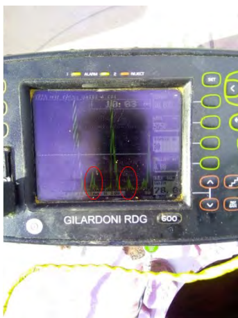
Figure 11 Critical area holder-reducer assessment of volume irregularities by conventional ultrasound method
