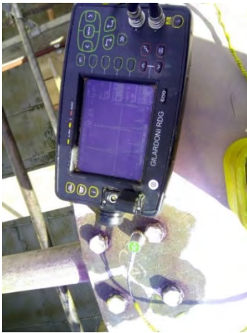
Figure 9 Critical place holder-blade evaluation of volume irregularity by using conventional ultrasonic method
