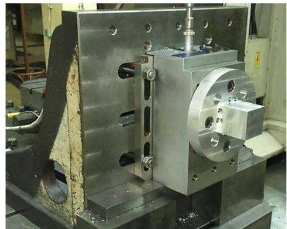
Figure 4. Machining on ILR HMC 500/40 [5]
