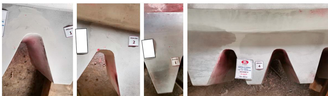
Fig. 5. Gear segments after polishing and no surface defects after PT.
