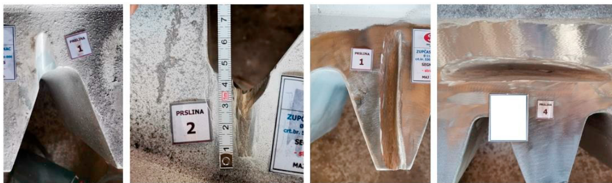
Fig. 2. Examples of prepared grooves on different gear segments.
