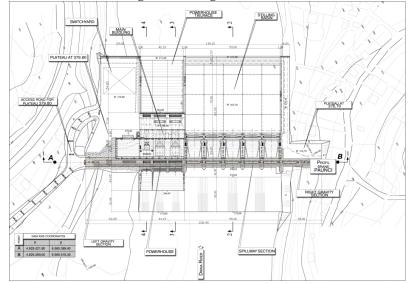
Hydropower facility consists of concrete overflow dam placed in the riverbed (Milosevic et al. (2013)). Normal water level is at 384.00 m, as well as the maximum water level, while the tail water level is at 379.51 m. Crest elevation is at 385.5 m, while the lowest foundation elevation (under the powerhouse) is 355.25 m. Powerhouse section is 52m long, while its width varies according to the tailrace width. Overflow section is 27m long, while its width is adjusted to the stilling basin width.
