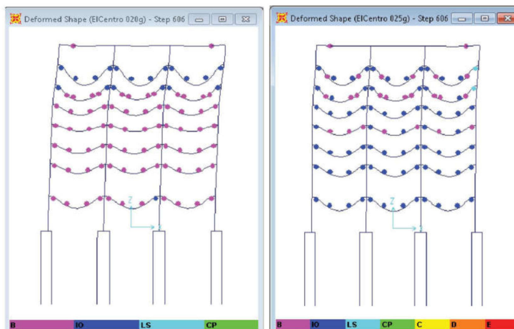
Figure 5. State of plastic hinges (PHS) at the end of earthquake El Centro, left PGA 0.20g PHS: 79Y, 19 IO; right PGA 0.25g PHS: 71Y, 25 IO and 2 LS. Linear roof beam
