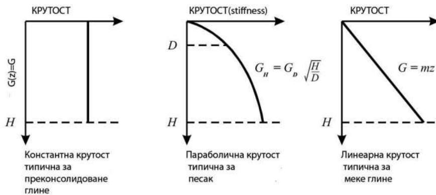
Slika 1 Raspodela krutosti po dubini profila tla: konstantna, parabolichna i linearna Figure 1 Distribution of stiffness along the depth of soil profile: constant, parabolic and linear
