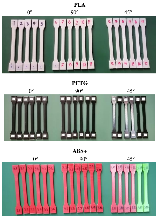
Fig. 6 Groups of printed out specimens, depending on material and printing orientation
