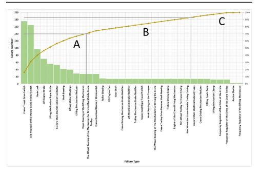
Figure 2: Pareto diagram of failures and stoppages for transport machinery.
