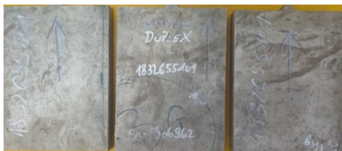
Figure 1. Delivered specimens of Super Duplex grade S32750.
