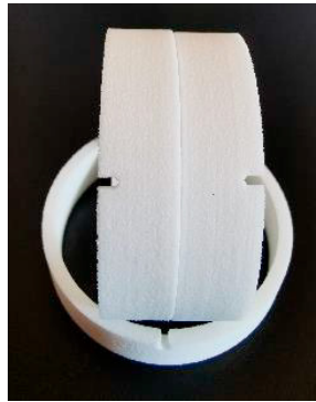
Fig. 2 PRNT specimens fabricated from PA12 material.
