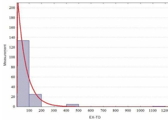
Figure 3. Histograms for failure/stoppage time of excavators
