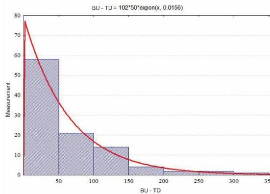
Figure 6. Histograms for failure/stoppage time of bulldozers
