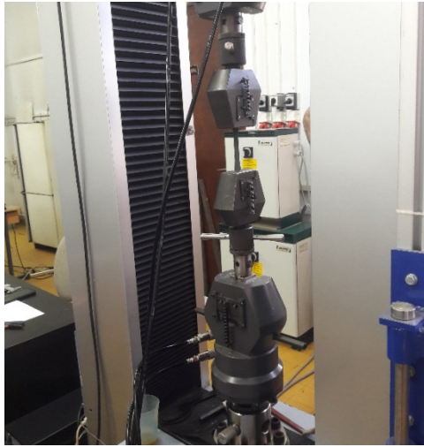
Fig. 4 Experimental setup used for the tensile test
