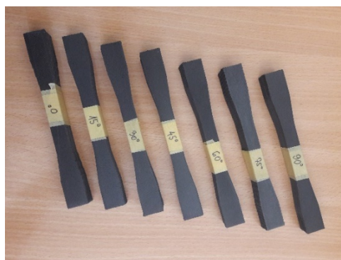
Fig. 3 Series of printed samples prepared for testing
