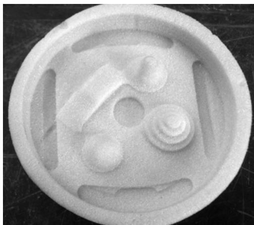
**Figure 6:** Device programming system. **Figure 7:** Test piece made of foam.
