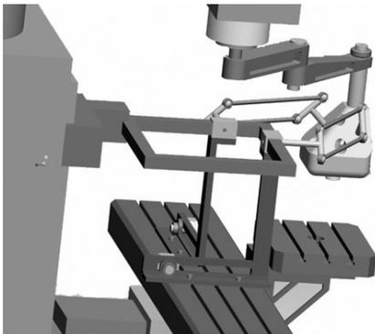
**Figure 9:** Hybrid device with SCARA mechanism.
