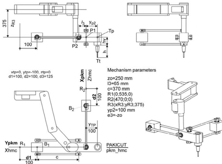
**Figure 14:** Structure of the hybrid device without own linear joints.
