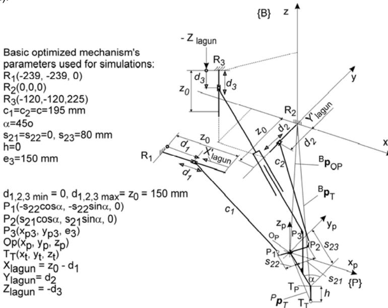
**Figure 12:** Geometric model of the devices shown in figures 9 and 10.
