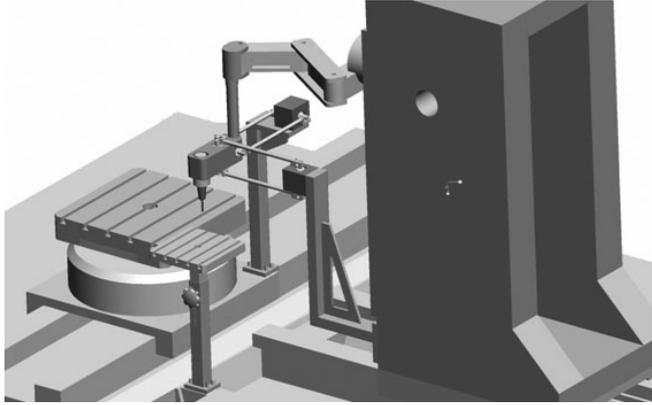
**Figure 11:** Hybrid device without own linear joints.
