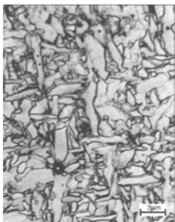
Fig. 4. Nucleation of AF on oxide inclusions. 12
