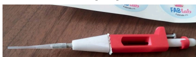
Figure 3 Prototype of a 3D printed micropipette produced in the SciFabLab in cooperation with PolyhedraFabLab
