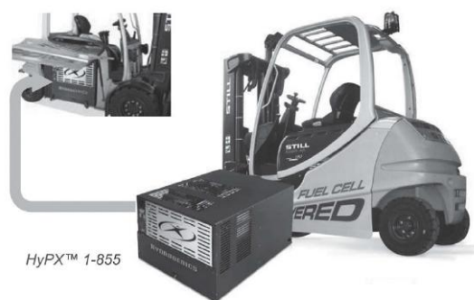
Figure 6. Still GmbH RX-60-45 forklift runs on HyPX 1-855 PEMFC from Hydrogenics [9]
