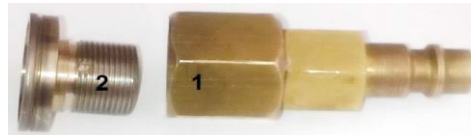
Fig. 3. Diaphragm test assembly: 1 quick coupling; 2 – body of measurement chamber with the diaphragm
