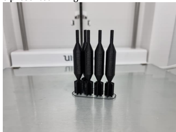
Figure 2: 3D printed projectiles
