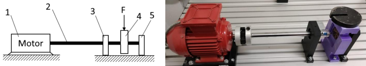
Fig. 2. Test bed for the gear bearing
