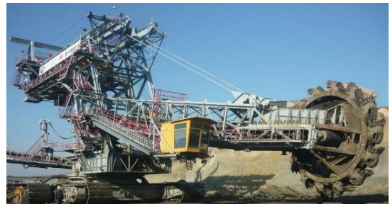
Fig. 1. Bucket wheel excavator SRs 1201
