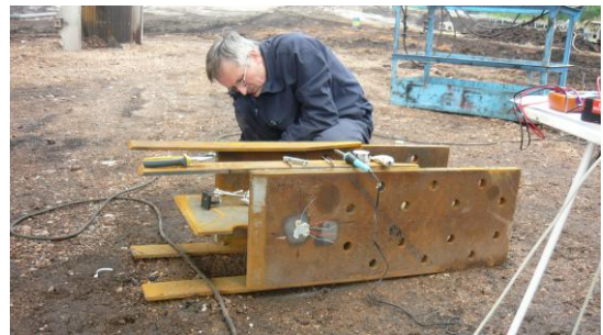
Fig. 14. Set up and connection of strain gauges
