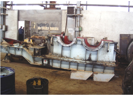
Figure 5. Lower part of the cover
