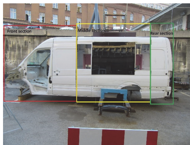
Figure 6 Body structure divided into three sections for the purpose of quasi-static loading test
