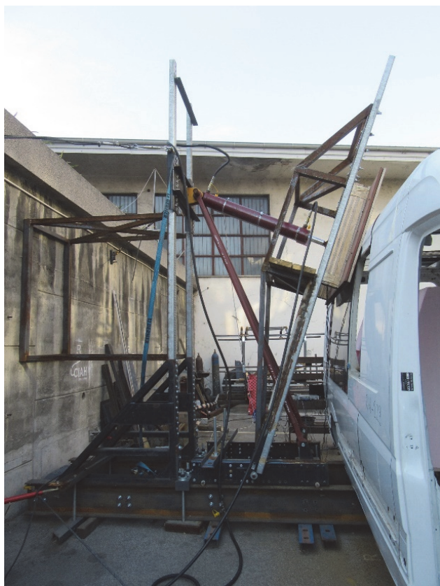
Figure 5 Test bench for physical tests according to UN Regulation No. 66
