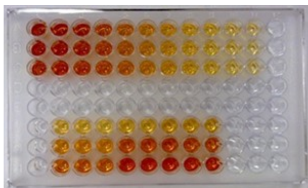
Fig. 5. An image of the assay plate of the proposed 96-microwell-based spectrophotometric assay of FQAs involving formation of CTC with DDQ. The plate contains the calibration solutions of varying drug concentrations (upper wells) and test samples (lower wells).
