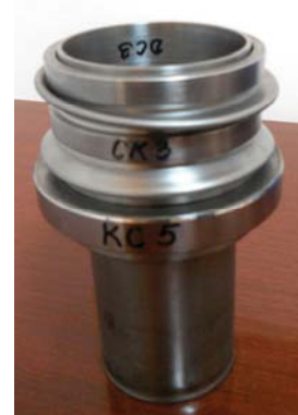
Fig.7. Combined absorber after experimental investigations – V = 25 mm/s
