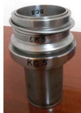
Fig.6. Deformed shrinking-folding absorber
