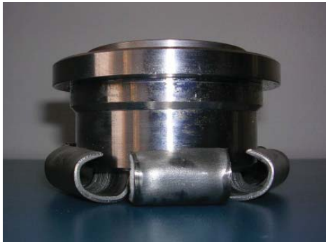
Fig. 8. Deformed shrinking-splitting absorber
