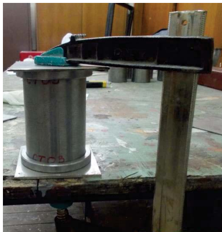
Fig.4. Filling the tube with foam
