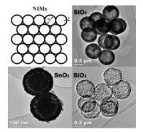
Figure 8. Conceptual model of silicon dioxide with holllow nanospheres [17].
