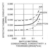
Figure 6: Effect of 1. number and thickness of buffles within GFP materials filled with argon; 2. different gasses within buffles on effective thermal conductivity [14].
