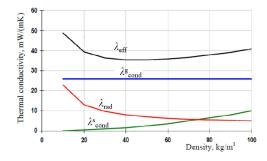
Figure 3. Influence of material density on mechanisms of heat transfer through porous microstructure [7].
