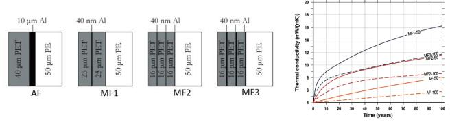
Figure 5. 1) Cross section of different configurations of vacuum insulation panels with barrier films made of alluminum films (AF) or metalized polymer films (MF) [9]; 2) Effect of panel size (50 cm x 50 cm x 1cm i 100 cm x 100 cm x 2cm) with different configurations of envelope (AF, MF1, MF2) on effective themrnal conductivity of VIP over time [4].
