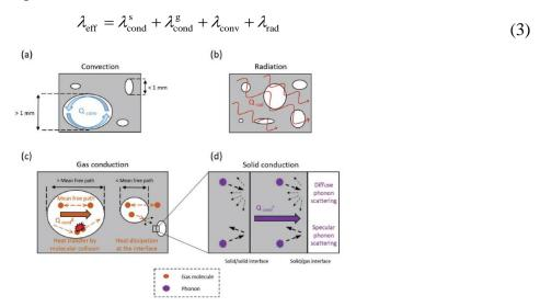
Figure 2. Schematic diagram of mechanisms of heat transfer through porous microstructure of construction materials [6].
