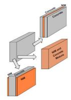
Figure 10. Different configurations of nano insulation materials and combinations with concrete [8].
