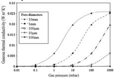
Figure 4. Change of gas thermal conductivity as a function of 1. achieved pressure within proes for different cores of material [9]; 2. achieved gas pressure and pores diameter [10].
