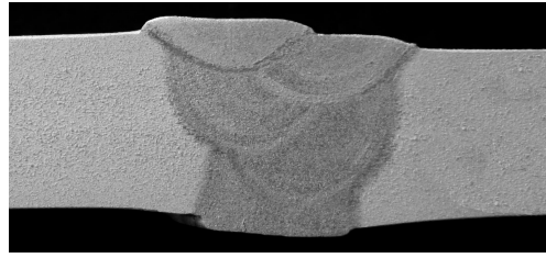
Figure 2. Macrograph of GTAW welded joint.
