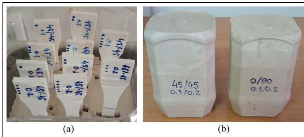
Figure 5. Specimen moulding in gypsum: (a) specimens were submerged and (b) mould formation before annealing.
