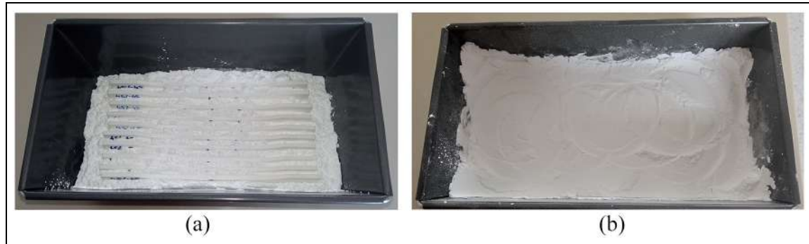
Figure 4. Specimen moulding in NaCl powder: (a) specimen drowning and (b) finished mould.
