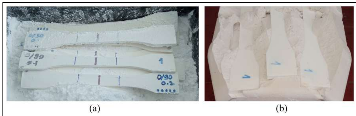
Figure 8. Specimens after removal from the mould: (a) NaCl powder and (b) gypsum.
